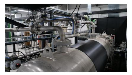
The system provides effective contact cooling of the pyrolysis gas, the removal of water, which is the product of the Sabatier reaction, prevents the formation of undesirable components of the gas mixture.
